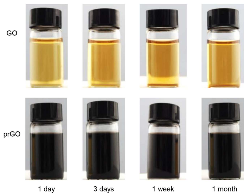
Figure S1. The as-prepared GO and prGO sheets are well dispersed in water for a long time.
