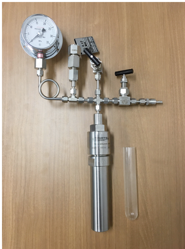
Figure S19. Photograph of a 100 mL-volume pressure-tight autoclave reactor (TPR6-VS2-100, Taiatsu Techno®) used for the perchlorination reaction of CB 11 H 12 - (1).
