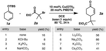
[a] Isolated yield from reaction of of dienol ether 1a (0.25 mmol),  $\alpha$ -haloester 2a (1.5 equiv), base (1.0 equiv), Cu(OTf)<sub>2</sub> (10 mol%), PMDTA (20 mol%) in 1 mL of DCE at 80 °C for 24 h.
