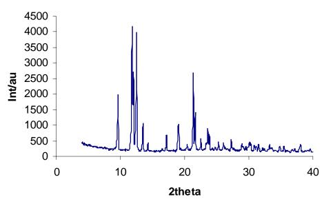
The observed pXRD pattern was taken after 5 days exposed to the atmosphere.
