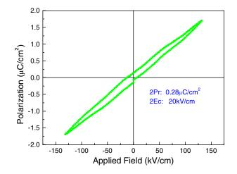
Figure 1S The electric hysteresis loop of **2** was observed by Virtual Ground Mode in a powdered sample in the form of a pellet using an RT6000 ferroelectric tester at room temperature
