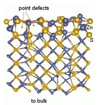
**Figure S.3** Side view of sphalerite Zn-rich (100) surface dynamically relaxed by MD at room temperature. The surface is relaxed both by relaxation (shortening in layer distance) and reconstruction (repositioning) of atoms. Point defects near the surface are created as a result of the reconstruction. (Bigger balls: atoms on or near the surface).
