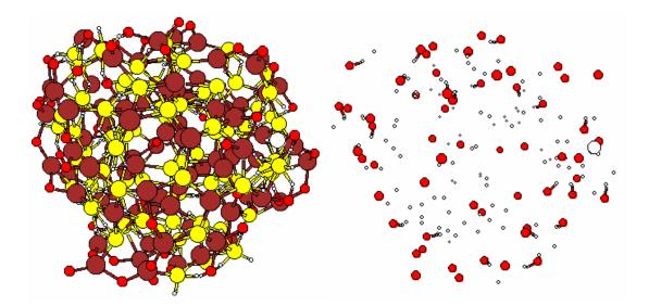
**Figure S.6** Equilibrated shape of the ZnS nanoparticle after adsorption of 61 CF water molecules (left). Adsorbed water molecules are shown on the right alone. The nanoparticle is slightly distorted. Water molecules are strongly dissociated. (Zn atoms are shown in brown, S in yellow, O in red and H in while circles).
