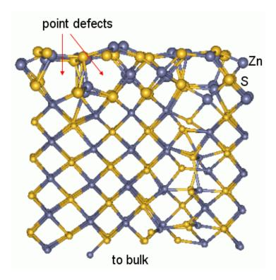
**Figure S.1** Side view of sphalerite S-rich (100) surface dynamically relaxed by MD at room temperature. The surface is relaxed both by relaxation (shortening in layer distance) and reconstruction (repositioning) of atoms. Point defects near the surface are created as a result of the reconstruction. (Bigger balls: atoms on or near the surface).
