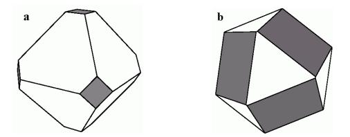
**Figure S.4.** Calculated morphology of a sphalerite crystal bounded by 6 {100} faces (shaded gray), 4 {111} faces and 4 {1  $\overline{11}$ } faces using surface energies from present work (a) or from ref.1 (b). The Wulffman program <sup>2</sup> was used in the calculation.
