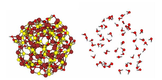
**Figure S.7** Equilibrated shape of the ZnS nanoparticle after adsorption of 61 shell model water molecules (left). Adsorbed water molecules are shown on the right alone. The nanoparticle essentially keeps the spherical shape. Water molecules are not dissociated. (Zn atoms are shown in brown, S in yellow, O in red and H in while circles).
