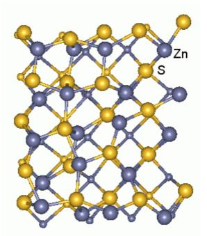
**Figure S.2** Top view of sphalerite S-rich (100) surface dynamically relaxed by MD at room temperature. Due to the reconstruction, surface atoms do not have exactly the same lattice arrangements as in the bulk. (Bigger balls: atoms on or near the surface).
