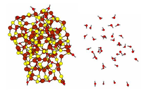
**Figure S.5** Equilibrated shape of the ZnS nanoparticle after adsorption of 40 SPCE water molecules (left). Adsorbed water molecules are shown on the right alone. The nanoparticle is highly distorted. Water molecules are not dissociated. (Zn atoms are shown in brown, S in yellow, O in red and H in while circles).
