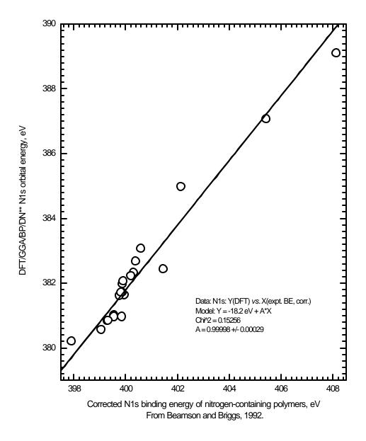
**Figure S1.** Correlation between the DFT N1s orbital energies (negative of the Kohn-Sham core-level energies) and the experimental N1s BEs of nitrogen-containing polymers. Identification of the models for polymer segments and data from Table S1.
