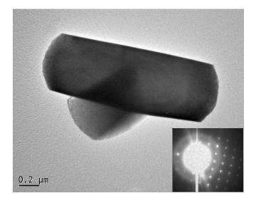
(ii) TEM images and ED pattern for [001] oriented anatase  $TiO_2$  crystallites (together with some bipyramidal microcrystals) grown without  $\alpha$ -MoO<sub>3</sub> template. Note that population of bipyramidal microcrystals has been significantly reduced. Experimental conditions: [TiF<sub>4</sub>] = 1.33 mM (30 mL), TiF<sub>4</sub>/EDTA molar ratio = 0.72; at 200°C for 5 h.
