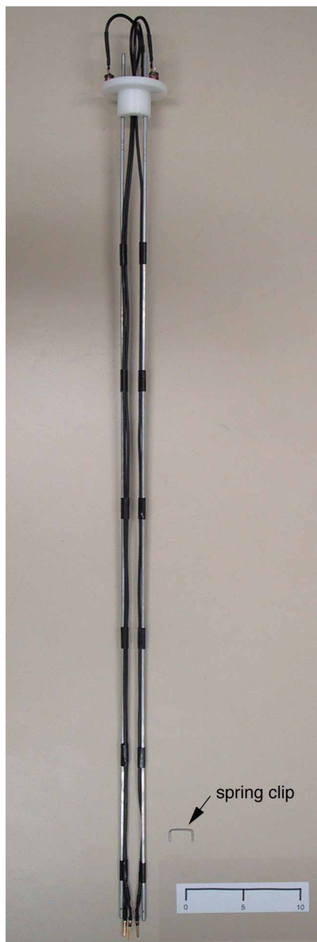
S-2.2. The aluminum rods were slid into holes in the Delrin block and held in place with screws in the side of the Delrin. The RF shielded wires were taped to the side of the aluminum rods, passed through a hole in the centre of the Delrin block and connected to the RF chokes. The RF chokes had two connections (going into and coming out of the coils), which allowed a convenient location to attach the wires from the potentiostat (see S-3.4).
