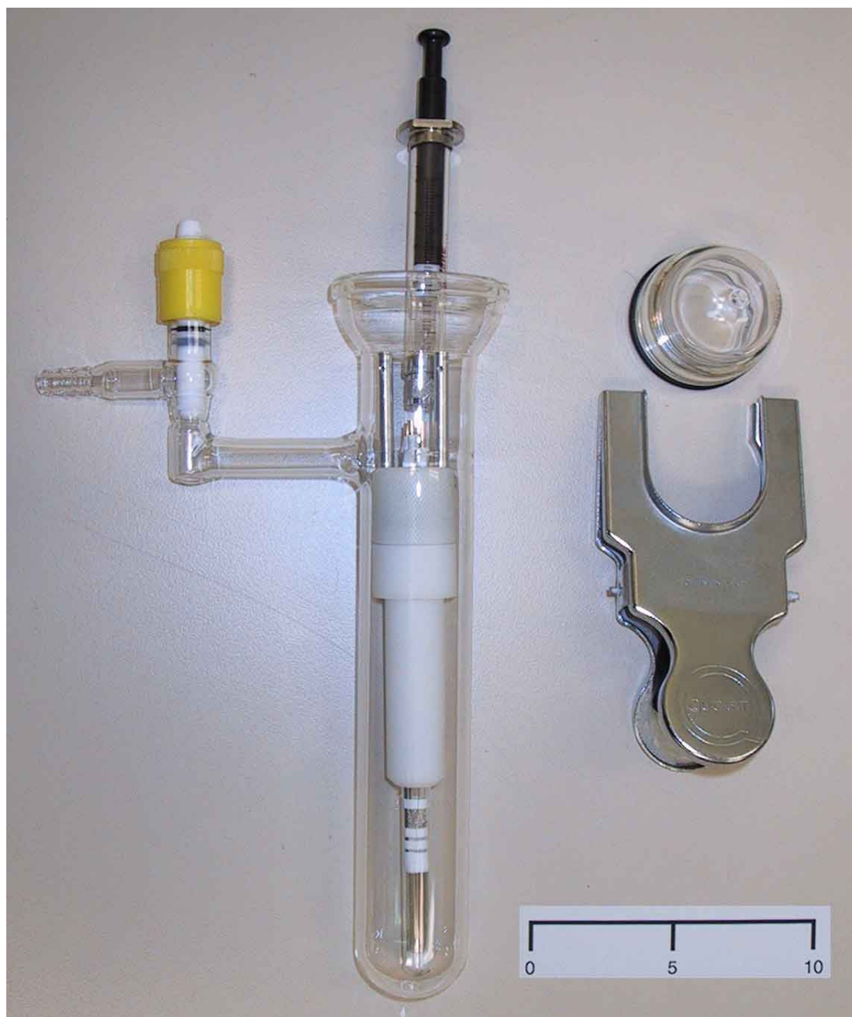
S-1.15. The assembled cell had a 3 mm diameter hole drilled in the Delrin lid that allowed it to be deoxygenated under vacuum in a Schlenk tube type apparatus and purged in a nitrogen atmosphere. The cell was filled with a deoxygenated solution via an airtight syringe through the 3 mm hole, which was sealed with a Teflon stopper. The filling solution passed through the frit at the base of the auxiliary electrode compartment before filling up the area surrounding the working electrode, with the process taking around 4-5 minutes. The total solution volume of the cell was ca. 2 mL. The volume of solution that resided between the 10 mm OD (9.07 mm ID) and 7.49 mm OD NMR tubes and within the RF coils inside the magnet was 0.33 cm 3 .
