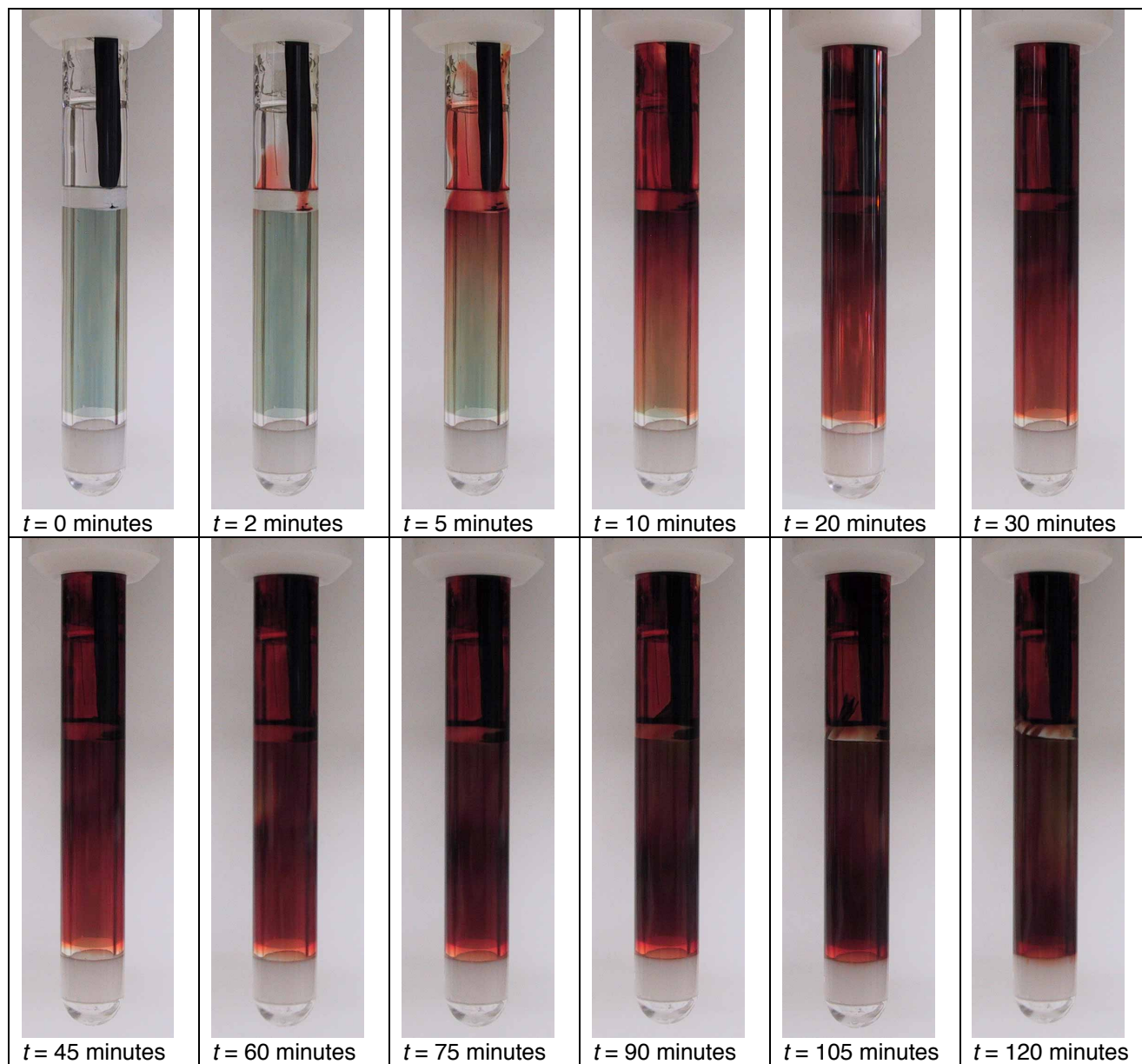
S-4.1. The photographs above show the constant potential one-electron reduction of 40 mM dimethyl pyridine-2,5-dicarboxylate in \text{CH}_3\text{CN} with 0.25 M \text{Bu}_4\text{NPF}_6 as the supporting electrolyte (Scheme 1). 2
