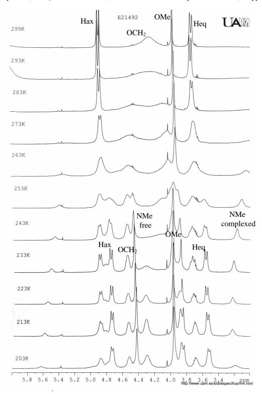
$^{1}$ H NMR spectrum (CDCl<sub>3</sub>/MeOD + 60% HNO<sub>3</sub>, 200 MHz, 298K) of compound **2** (0.50-9.00 ppm)
