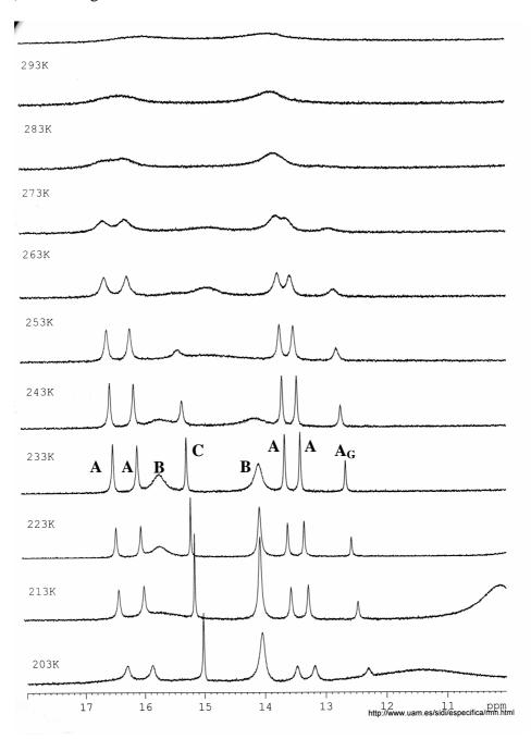
$VT^{-1}H$  NMR spectra (CDCl<sub>3</sub> + TFA, 500 MHz) of a 1:1 mixture of compounds **2** and **6** (3-6 ppm).
