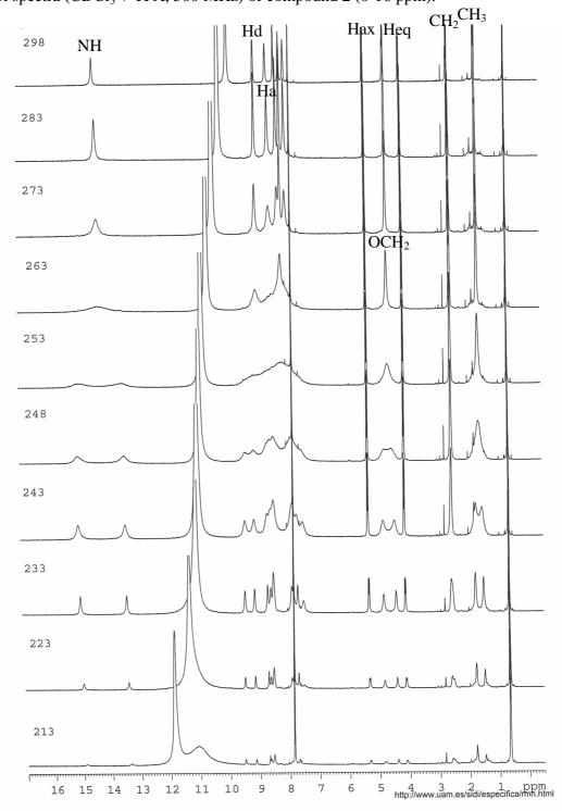
VT-<sup>1</sup>H NMR spectra (CDCl<sub>3</sub> + TFA, 500 MHz) of a 1:1 mixture of compounds **2** and **6** (10-18 ppm). **A**: NHs signals of complexed **2** (*pinched cone*); **A**<sub>G</sub>: NH signal of complexed **6**; **B**: NH signal of free **2** (*pinched cone*); **C**: NH signal of free **6**.
