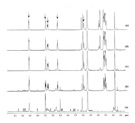
2) Pseudorotaxane formation ( $\downarrow$ , 300 MHz) by the the addition of  $\gamma$ CD to the macrocyclic complex **M'** (0.1 mM) derived from Pd(1,2-diaminocyclohexane) in D<sub>2</sub>O, according to the equivalents of the  $\gamma$ -CD added (a) 0 equiv, (b) 4 equiv.
