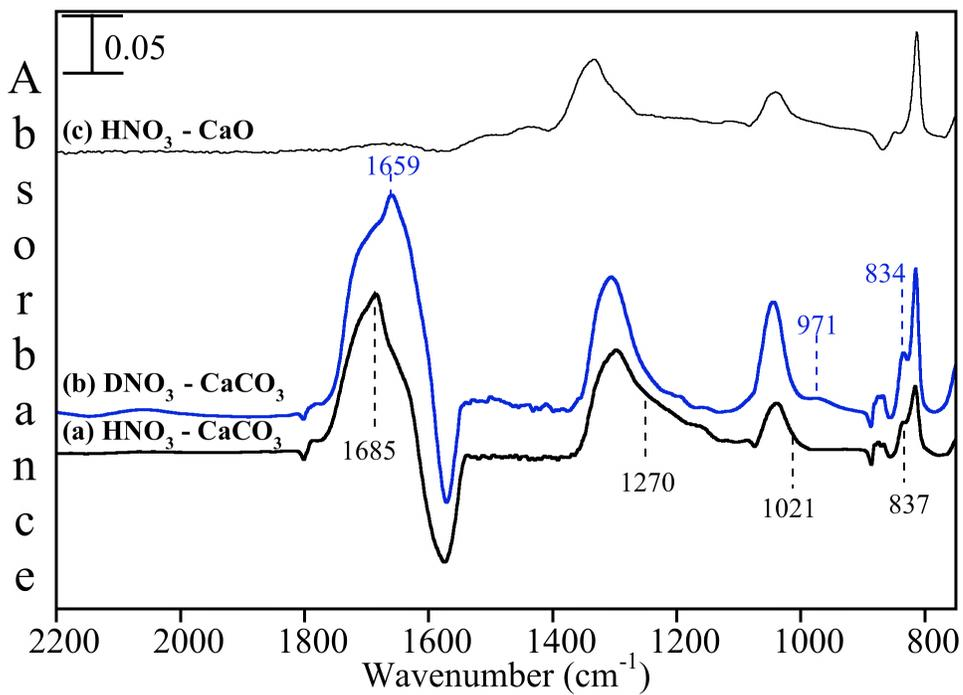
**Supplemental Figure 1.** (a) Adsorption of  $\sim 150$  mTorr of  $\text{HNO}_3$  on  $\text{CaCO}_3$ . (b) Adsorption of  $\sim 150$  mTorr  $\text{DNO}_3$  on  $\text{CaCO}_3$  pretreated with  $\text{D}_2\text{O}$ . (c) Adsorption of  $\sim 150$  mTorr  $\text{HNO}_3$  on  $\text{CaO}$ . Frequencies of adsorbed  $\text{H}_2\text{CO}_3$  and  $\text{D}_2\text{CO}_3$  are labeled in the figure. All other absorption bands are associated with adsorbed nitrate ions.
