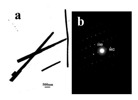
**Figure 3S**. TEM image (a) and corresponding ED pattern (b) of the thinner ZnO nanorods in sample 4.
