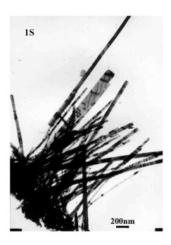
Figure 1S. TEM image of ZnO nanorod array in Sample1.
