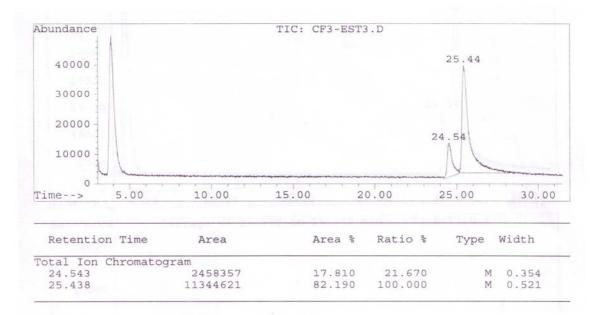
For compound 4c.  $\beta$ -DEX<sup>TM</sup> column (30 m × 0.25 µm); T= 110 °C isotherm. Tdet. = Tinlet = 225 °C;
