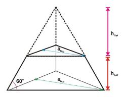
The parameters are defined as follows:  $a_{bot}$  is the in-plane width of the nanoparticle,  $h_{bot}$  is the out-ofplane height of the nanoparticle,  $h_{top}$  is the height of the top of the tetrahedron not including the volume
