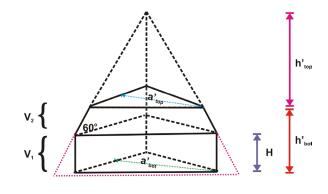
The parameters in these expressions are defined as follows:  $a_{bot}$  is the in-plane width of the nanoparticle (also the width of the trigonal prism),  $h_{bot}$  is the out-of-plane height of the nanoparticle,  $h_{top}$  is the height of the top of the tetrahedron not including the volume taken up by the particle,  $a_{top}$  is the in-plane width of the top volume of the tetrahedron, and *H* is height of the trigonal prism.
