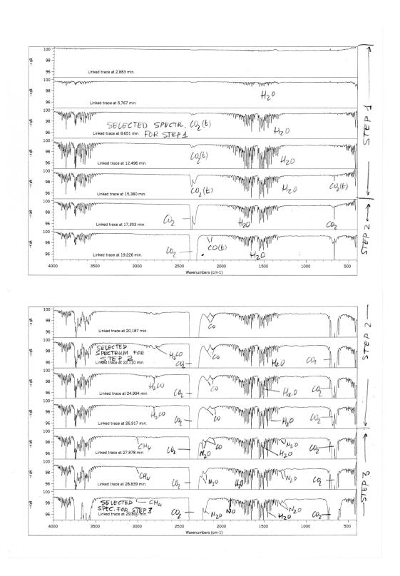
S1C (cont). FT-IR spectra recorded during the TG analysis of compound 1-o. On the right-hand is indicated the 5 or 6 spectra corresponding to each step. Four of these spectra (one per step) were selected as is shown in S1E.
