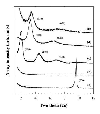
**S2**. Powder XRD patterns for microporous nanohybrid derivatives: (a) layered titanate, (b) the colloidal suspension of exfoliated titanate, (c) as-prepared microporous nanohybrid, (d) microporous nanohybrid with the heat-treatment at  $300\,^{\circ}$ C, (e) microporous nanohybrid with the heat-treatment at  $350\,^{\circ}$ C.
