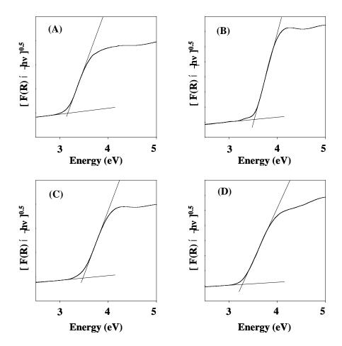
**S1**. Plots of [  $F(R) \times hv$  ]<sup>0.5</sup> vs energy, where R is the reflectance from the UV-vis diffuse reflectance measurements: (A)  $TiO_2$  xerogel,  $E_g = 3.2$  eV: (B) layered cesium titanate,  $E_g = 3.5$  eV: (C) layered protonic titanate,  $E_g = 3.4$  eV: (D) nanohybrid-I,  $E_g = 3.3$  eV. The intercept of the two linearly extrapolated lines gives the bandgap energy  $(E_g)$ .
