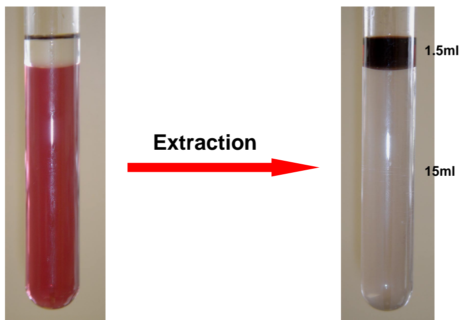
Figure S3: Digital images illustrating the effective extraction of Au nanoparticles from an aqueous \beta -D glucose solution into a hexane phase via ligand exchange from \beta -D glucose to dodecanethiol. These images display the generation of highly concentrated dodecanethiol capped Au nanoparticle dispersions in hexane.
