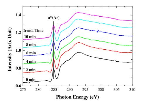
**S1.** Series of carbon K-edge NEXAFS spectra of benzaldimine monolayer irradiated by 500 eV electron beam. Each spectrum is subtracted by the spectrum of a bare silicon surface to remove substrate contribution.
