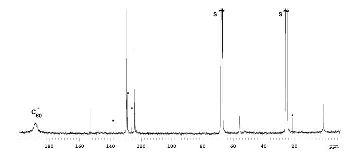
**Figure S2**. <sup>13</sup>C NMR of **2** in d8-THF. The peaks labelled with asterisk are due to toluene.
