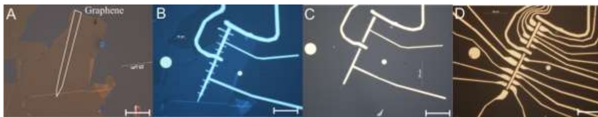
Figure S10. Schematic of the fabrication process for devices encapsulated with micro mechanically exfoliated h-BN (MME-h-BN) (a) mechanically exfoliated h-BN crystal used to lift exfoliated graphene from \text{SiO}_2 substrate. (b) The \text{Al}_2\text{O}_3 / EM -h-BN / MME graphene / MME-h-BN stack with added Au gate electrodes (50 nm) and Aluminum etch mask. (c) the structure after etching away MME-h-BN in a Freon plasma. (d) 1D contacts added to the MME-graphene encapsulated between EM -h-BN and MME-h-BN (Scale bar = 20 \mu\text{m} ).
