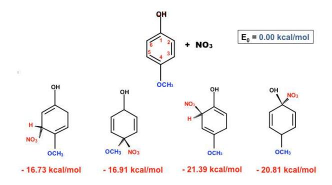
Figure S8. Relative stability,  $\Delta E_0$ , of the adducts formed from the reaction of 2-M-4-MeP with nitrate radicals (calculation done using DFT: UM06-2X/6-31G(d,p)).
