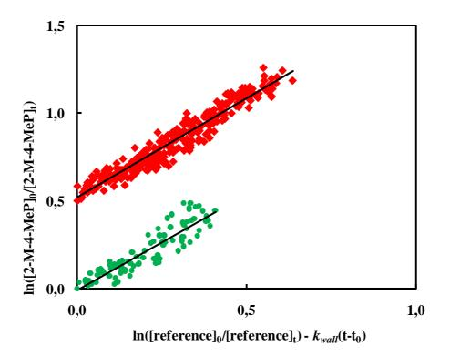
Figure S4. Kinetic data plot for the reaction of syringol (2,6-DMP) with nitrate radicals at  $(294 \pm 3)$  K using catechol (•) and 3-methylcatechol (•) as reference compounds. For clarity, data obtained with catechol have been vertically shifted by 0.5 units. The organic compound concentrations were monitored with PTR-ToF-MS.
