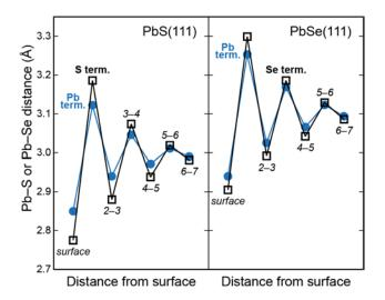
**Figure S2** (*as supplement to Figure 3 in the main text*): Course of Pb–S and Pb–Se bond lengths near the relaxed, pristine (111) surfaces. Results at the PBE level of theory are shown.
