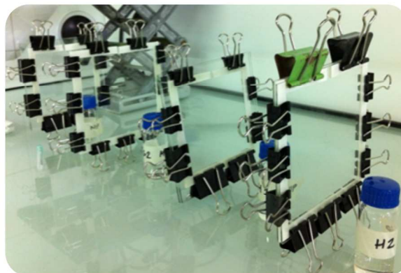
Figure S2. Scheme of the polymerization molds used for the films preparation. The glass slides ( 10 \times 10 cm) were separated by a 0.9 mm thick silicone gasket (1 cm wide), compressed to create a leak-free seal and filled in with the prepolymerization mixture.
