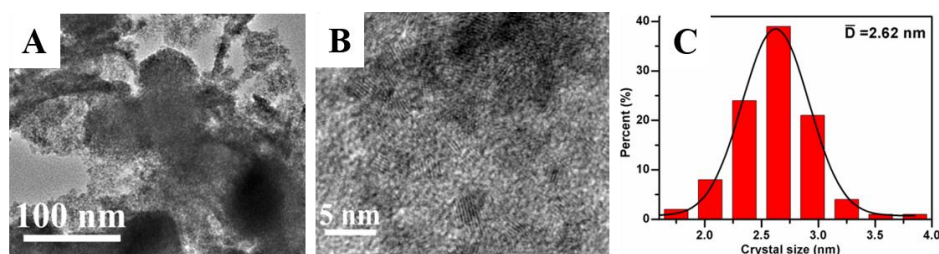
Figure S2. HRTEM (A and B) images and crystal size distribution (C) of SnO 2 -200-0.25.
