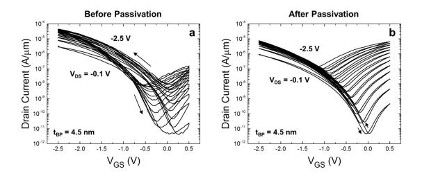
Figure S4. Double sweep transfer characteristic of device #3 (a) before and (b) after passivation for values of  $V_{DS} = -0.1$  to -2.5 V in -0.2 V steps. Possible causes for the hysteresis include charge trapping in the HfO<sub>2</sub> gate dielectric, moisture trapped underneath the BP, and/or surface oxide layers on top of the BP. The hysteresis was greatly reduced after passivation, which we attribute to moisture desorption during the passivation layer deposition step at 200°C.
