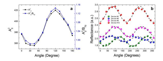
Figure S3. (a) Angular dependence of the Raman  $A_g^2$  mode (left axis) and  $A_g^2/B_{2g}$  (right axis) for a typical BP flake. The peak intensity is the direction that the laser polarization is along the armchair (low mass) direction. (b) Reflectance intensity as a function of rotational angle for devices #5, 8, 9, and 10. The maximum peak intensity indicates the zigzag direction (high mass). Dashed lines shows the sinusoidal fit of the reflectance data.
