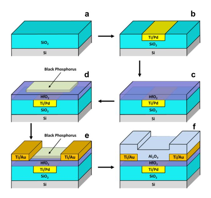
Figure S1. Fabrication sequence for BP MOSFETs. (a) Si/SiO<sub>2</sub> starting substrate, (b) local back gate formation, (c) ALD HfO<sub>2</sub> deposition, (d) black phosphorus alignment and transfer, (e) source and drain contact formation, (f) ALD Al<sub>2</sub>O<sub>3</sub> passivation layer deposition.
