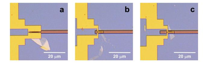
Figure S2. Optical micrographs of several completed BP MOSFETs. (a) Device #2 with BP thickness (in the active device region),  $t_{BP}$  of 4.3 nm. The device width,  $W_g$  was 7.15 µm and the source-to-drain spacing, which defined the effective gate length,  $L_{eff}$  was 1.0 µm. (b) Device #3 with  $t_{BP} = 4.5$  nm,  $W_g = 2.00$  µm and  $L_{eff} = 0.4$  µm, and (c) Device #7 with  $t_{BP} = 8.1$  nm,  $W_g = 3.16$  µm and  $L_{eff} = 0.30$  µm.
