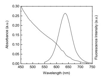
Figure S1. Absorption and emission spectra of CdTe nanocrystals in water.  $\lambda_{ex}$  = 470 nm.
