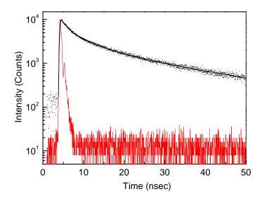
Figure S2. Intensity time decay of CdTe nanocrystals in water. Instrument response function is also included.
