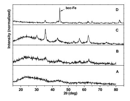
**Figure S3.** XRD patterns of (A) the as-synthesized 4-nm/2.5-nm Fe/Fe<sub>3</sub>O<sub>4</sub> nanoparticles, (B) the 2.5-nm/5-nm Fe/Fe<sub>3</sub>O<sub>4</sub> nanoparticles from controlled oxidation of the as-synthesized Fe nanoparticles, (C) oxidation of the as-synthesized Fe nanoparticles with excess of  $(CH_3)_3NO$ , and (D) the 2.5-nm/5nm Fe/Fe<sub>3</sub>O<sub>4</sub> nanoparticles annealed under Ar at 400°C for 1 h.
