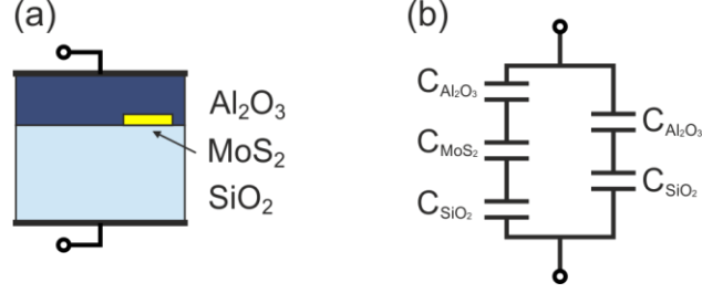
SI Figure 2. (a) Theoretical device structure. Two stacking areas of \text{Al}_2\text{O}_3/\text{MoS}_2/\text{SiO}_2 and \text{Al}_2\text{O}_3/\text{SiO}_2 sandwiched between two metallic plates. (b) Corresponding circuit diagram of the capacitor.
