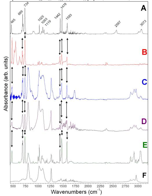
FTIR Spectra of  $TOA_{Z}[Au_{x}(SPh)_{y}]^{Z}$ ,  $(AuSPh)_{x}$  polymer, benzenethiol, and TOABr
