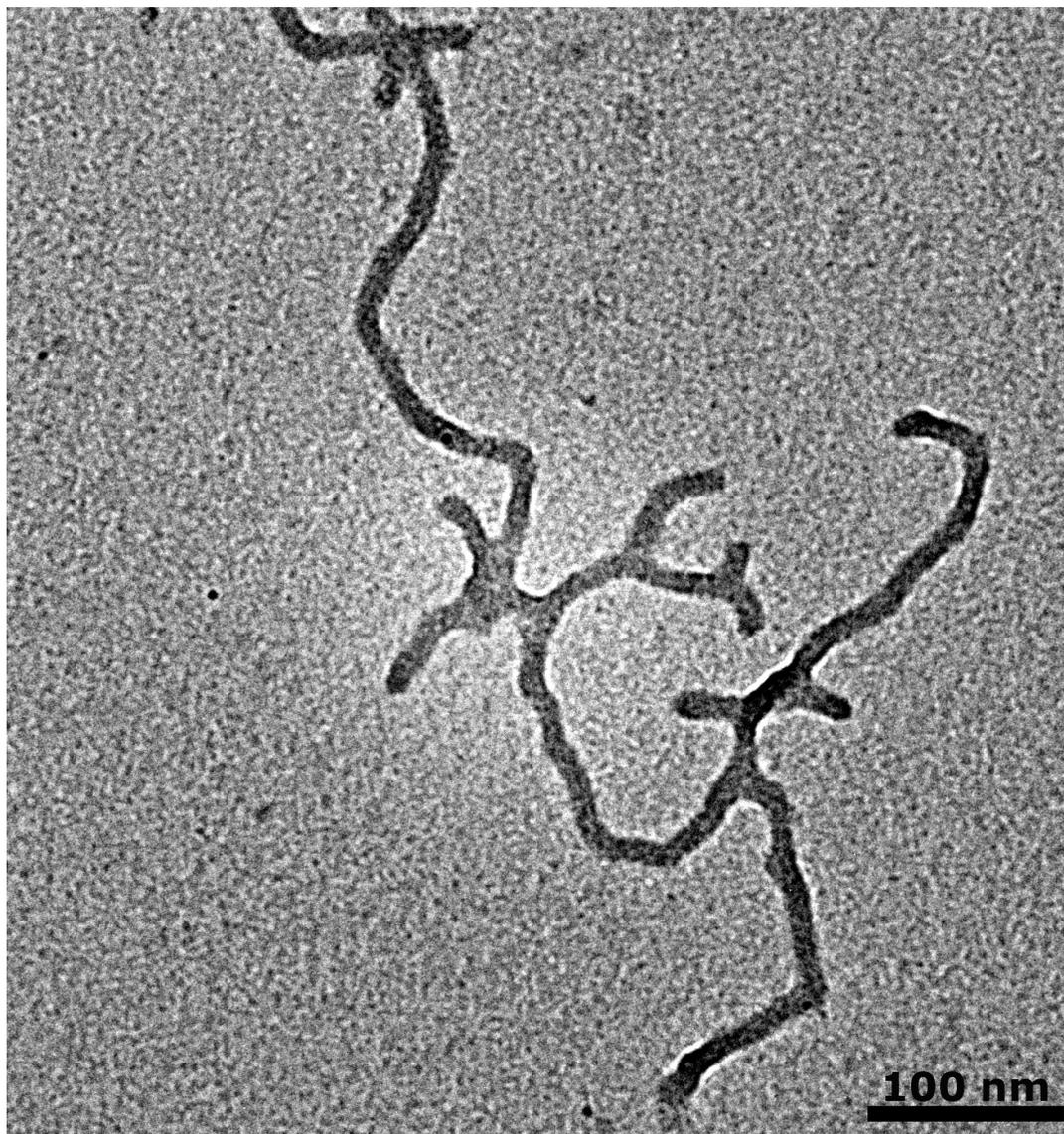
**Figure S7.** TEM images of worm-like assemblies of amphiphilic Au-(PS<sub>30</sub>-PEO<sub>50</sub>)<sub>n</sub> NPs from an aqueous solution after dialysis from a DMF/H<sub>2</sub>O (1:3 vol.) mixture. Please note the reduction in the diameter of the hydrophobic PS core from  $18 \pm 2$  nm (Fig. 1B in the text) to  $14 \pm 2$  nm as the molecular weight of the PS arms is decreased from 4,000 to 3,000 g/mol, respectively.
