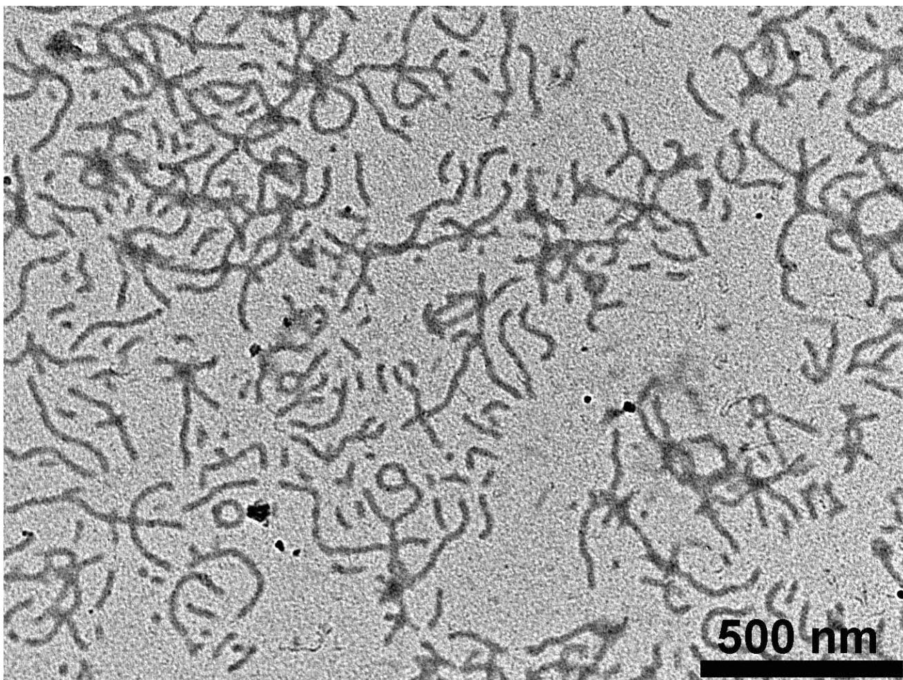
**Figure S3.** Unstained TEM image of structures from the aqueous solution of  $\text{Ag}(\text{PS}_{40}\text{-PEO}_{50})_n$  particles. A solution of  $\text{Ag}(\text{PS}_{40}\text{-PEO}_{50})_n$  in DMF/ $\text{H}_2\text{O}$  mixture was dialyzed against DI water for 3 days.
