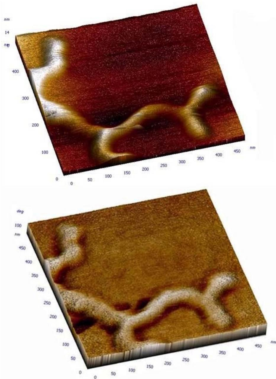
**Figure S4.** Topography (top) and phase contrast tapping mode AFM 3D images ( $500 \times 500$  nm) of structures formed by  $\text{Au}(\text{PS}_{40}\text{-PEO}_{50})_n$  in water (dialysis from DMF/ $\text{H}_2\text{O}$  mixture). Please note that the diameter appears to be  $\sim 50$  nm, which is significantly larger than that observed in TEM (18 nm). This is due to the tip dilation effect and the presence of PEO corona that is not visible in TEM images.
