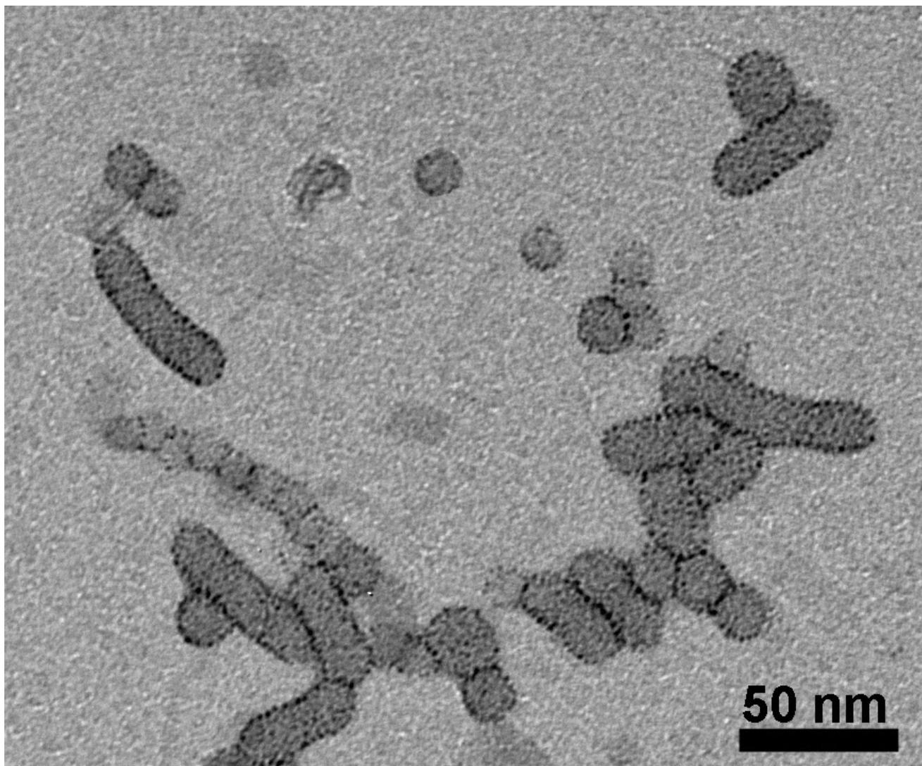
**Figure S8.** TEM images of short cylindrical and spherical assemblies of amphiphilic Au-(PS<sub>40</sub>-PEO<sub>50</sub>)<sub>n</sub> NPs from an aqueous solution containing 10 % (vol.) methanol. The sample was not stained, and the contrast was due to the gold core of the amphiphilic Au-(PS<sub>40</sub>-PEO<sub>50</sub>)<sub>n</sub> structures.
