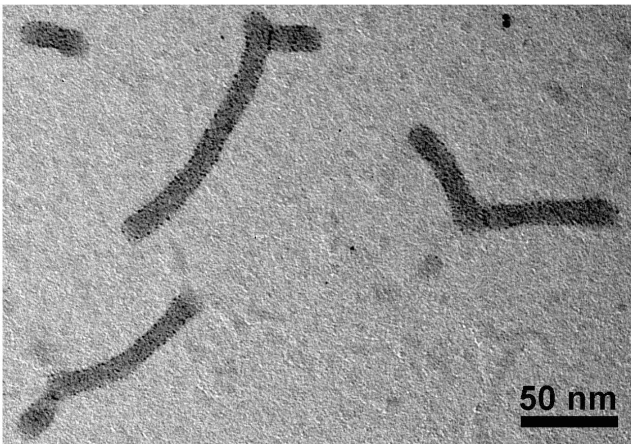
**Figure S2.** Unstained TEM image of structures from the aqueous solution of  $\text{Ag}(\text{PS}_{40}\text{-PEO}_{50})_n$  particles. A solution of  $\text{Ag}(\text{PS}_{40}\text{-PEO}_{50})_n$  in THF/ $\text{H}_2\text{O}$  mixture was dialyzed against DI water for 3 days.
