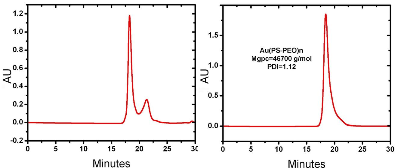
**Figure S1.** GPC trace of Au(PS<sub>40</sub>-PEO<sub>50</sub>)<sub>n</sub> nanoparticles. Left trace is taken from the reaction mixture before purification (small low molar mass peak corresponds to excess PS<sub>40</sub>-*b*-PEO<sub>50</sub> amphiphile **1**). Right GPC trace is taken after 3 rounds of centrifugal ultrafiltration (THF, 30 kDa MWCO membrane).
