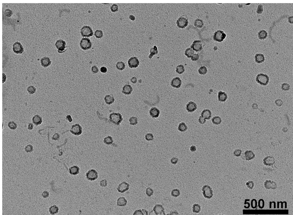
**Figure S9.** High (top) and low magnification TEM images of vesicular assemblies of amphiphilic Au(PS<sub>40</sub>-PEO<sub>50</sub>)<sub>n</sub> NPs from an aqueous solution prepared after dialysis from a concentrated solution (40 mg/mL) of Au(PS<sub>40</sub>-PEO<sub>50</sub>)<sub>n</sub> NPs in DMF.
