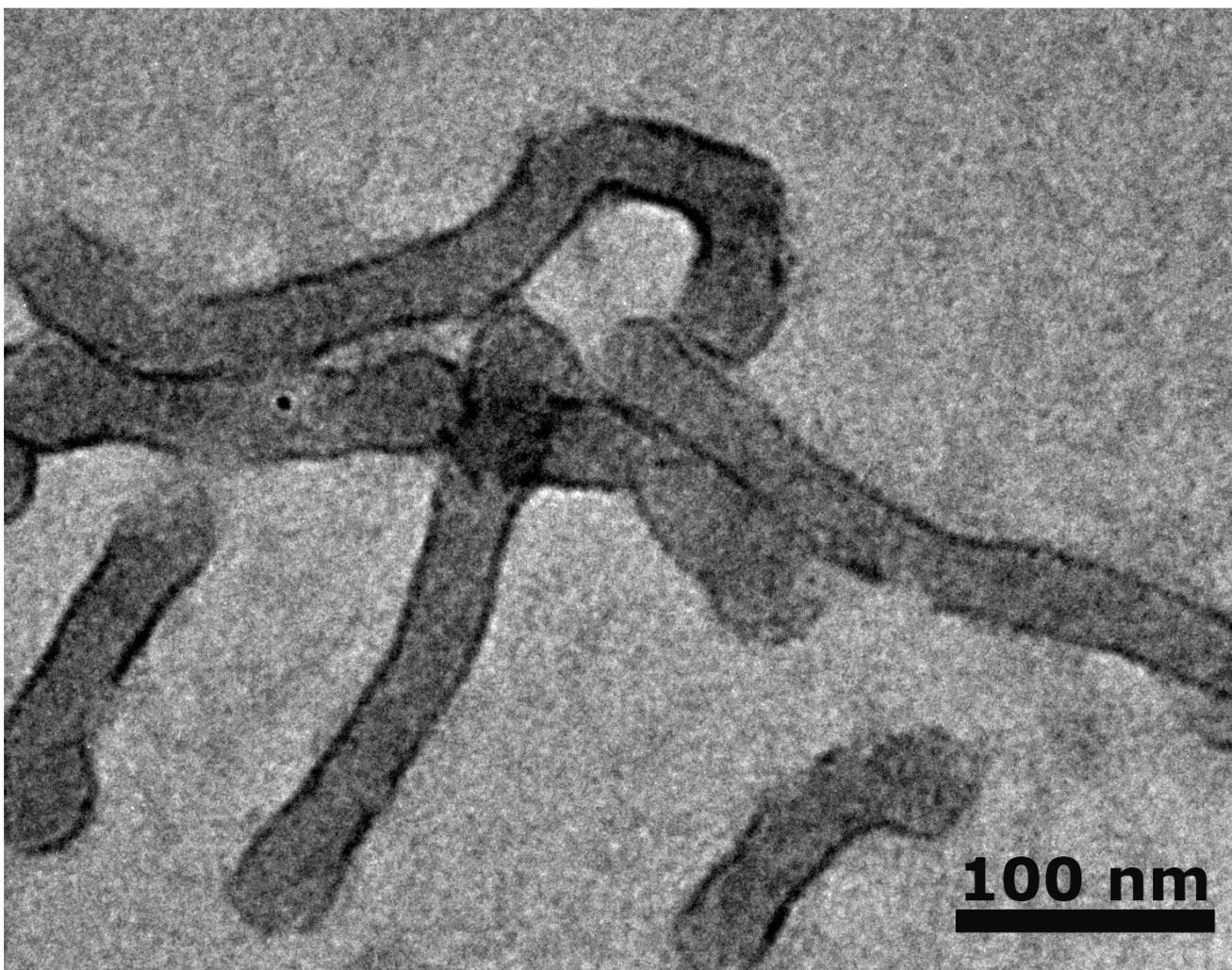
**Figure S10.** TEM images of worm-like assemblies of the amphiphilic Au-(PB<sub>100</sub>-PEO<sub>115</sub>)<sub>n</sub> NPs from an aqueous solution after the dialysis from a DMF/H<sub>2</sub>O (1:3 vol.) mixture. Please note the increase in the diameter of the hydrophobic core from  $18 \pm 2$  nm (Fig. 1B in the text) to  $32 \pm 3$  nm as the contour length of the hydrophobic arms is increased from  $\sim 10$  nm to  $\sim 50$  nm, respectively.
