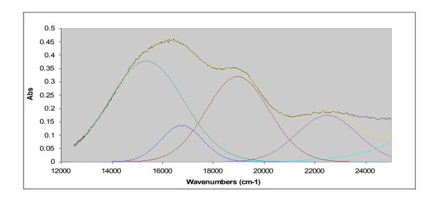
Figure S2. Absorbance spectrum of (2), fitted this way based on unpublished rR results.
