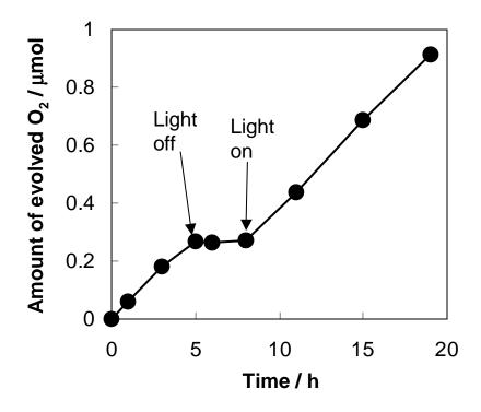
Figure S1: The reaction time profile of the photocatalytic evolution of  $O_2$  from a 0.05 M AgNO<sub>3</sub> aqueous solution on Pt-loaded N-TiO<sub>2</sub>(4) under visible light irradiation ( $\lambda \ge 420$  nm).
