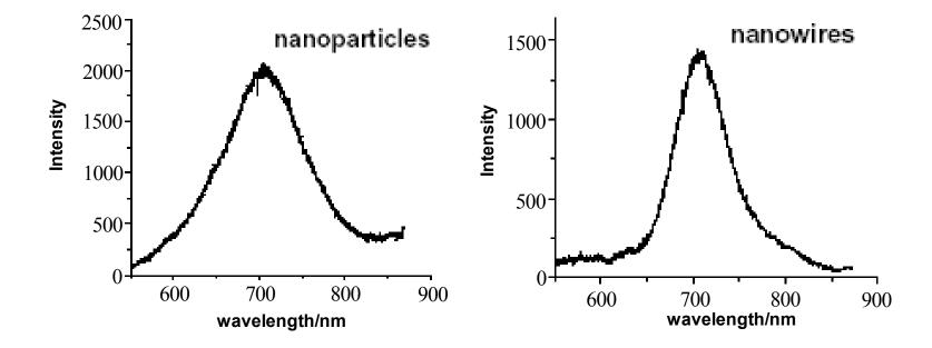
PL spectrum of nanoparticles obtained after one wetting cycle (FWHM ~ 80 nm,  $\lambda_{max}$  corresponds to the bulk bandgap)
