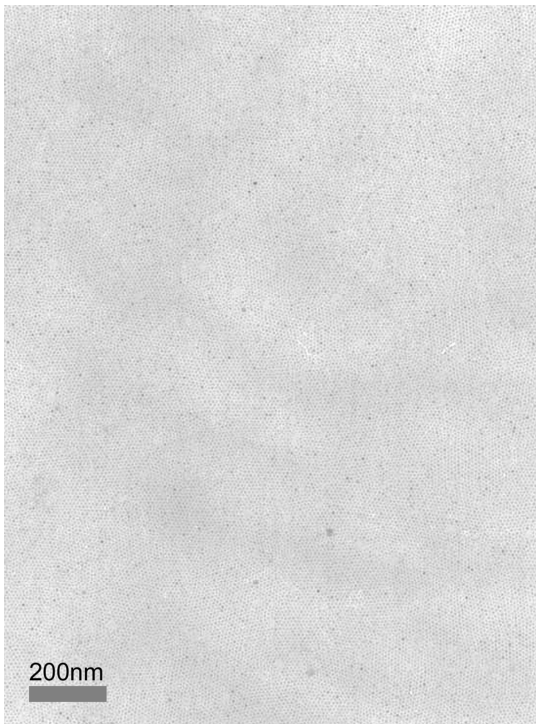
Figure S2 Large area TEM image of ZnS 2D NCAs (monolayer) prepared with PEG and oleylamine.
