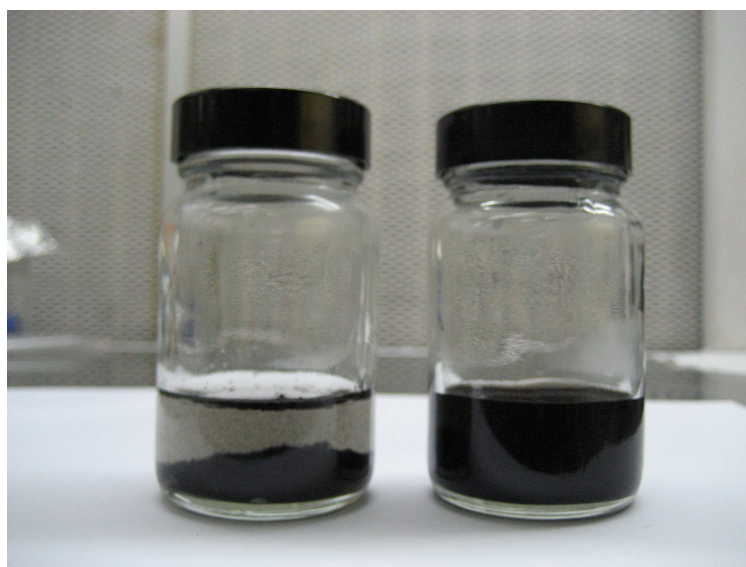
Figure S1. Optical micrographs of the pristine MWNTs (8 mg) were dispersed in 20 mL of HCl solution (pH=2.6) after standing for 1h (left) and the oxidized MWNTs (8 mg) were dispersed in the same solution after standing for one month (right).
