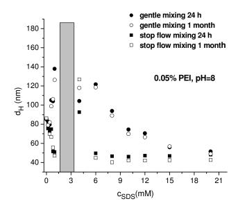
S4 Effect of time on the apparent hydrodynamic diameter of the PEI/SDS complexes. The squares and circles indicate the experimental results of the stop flow and the gentle mixing protocol, respectively. The solid and open symbols denote those data where the solutions were left to stand for 24 hours and 1 month, respectively after the preparation. pH=8, 0.05% PEI without added salt.
