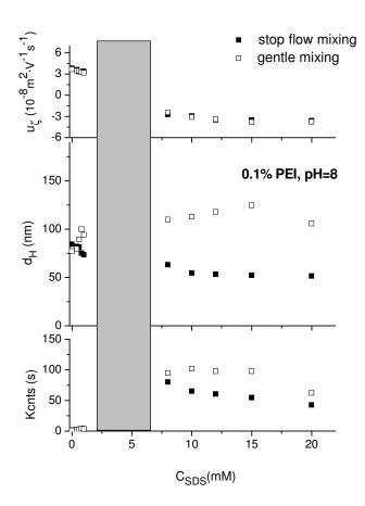
S2 The electrophoretic mobility and apparent hydrodynamic diameter of the PEI/SDS complexes as well as the intensity of the scattered light as a function of surfactant concentration for the two mixing protocols. Prior to the measurements the PEI/SDS solutions, prepared by the two methods, were left to stand for 24 hours. The gray area indicates the precipitated or the highly turbid systems. pH=8, 0.1% PEI without added salt.
