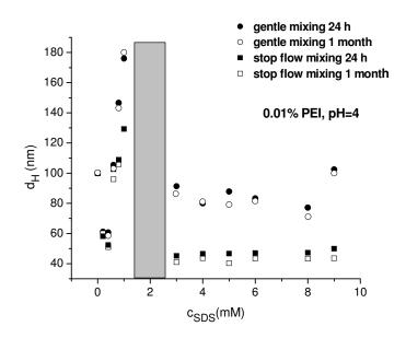
S3 Effect of time on the apparent hydrodynamic diameter of the PEI/SDS complexes. The squares and circles indicate the experimental results of the stop flow and the gentle mixing protocol, respectively. The solid and open symbols denote those data where the solutions were left to stand for 24 hours and 1 month, respectively after the preparation. pH=4, 0.01% PEI without added salt.
