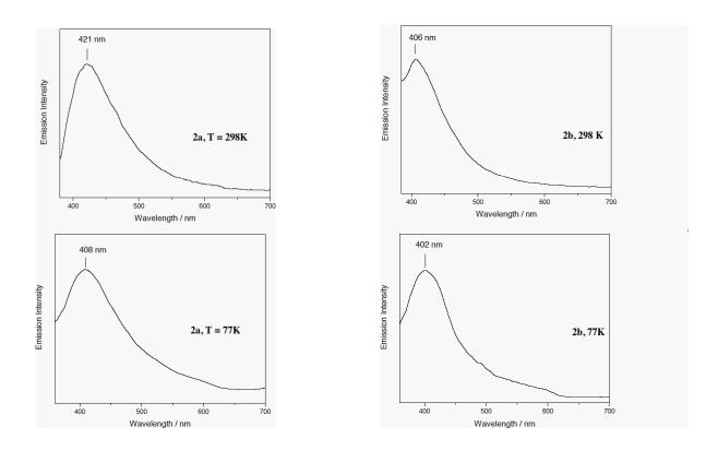
Figure S. Photoluminescene spectra of complexes **2a**, **b** at room temperature and at 77K with  $\lambda$  excitation around 330 to 350 nm.
