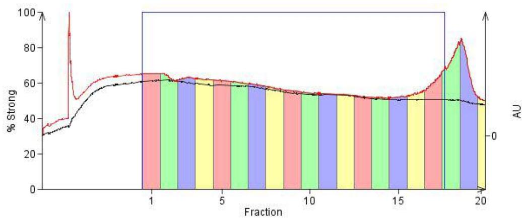
breakthrough curve of Pd(OAc)<sub>2</sub> in THF (1000 ppm) through QuadraPure TU cartridge
