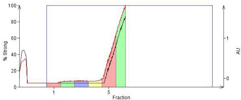
breakthrough curve of Cu(acac)<sub>2</sub> in DCM (1000 ppm) through QuadraPure IDA cartridge
