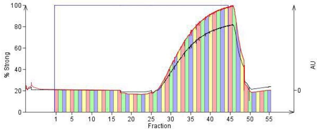
breakthrough curve of  $\text{FeCl}_3$  in THF (500 ppm) through QuadraPure AMPA cartridge
