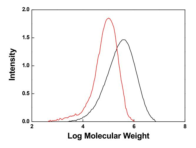
**Figure S1.** GPC curves for the PEs having the higher (black) and lower MW materials (red) used in this study. These curves were recorded in a solvent of 1,2,4 trichlorobenzene at Tosoh (Yokkaichi, Japan) using standard methods.
