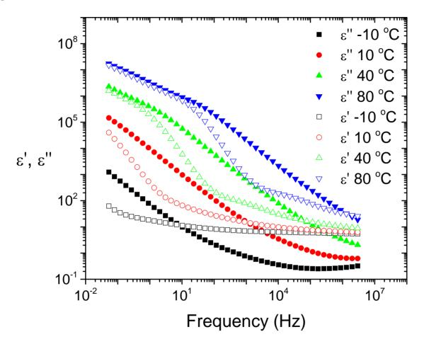
Dielectric constant and loss as a function of frequency across the temperature range of interest, for the ionomer with 17 mol % ions (I-17).
