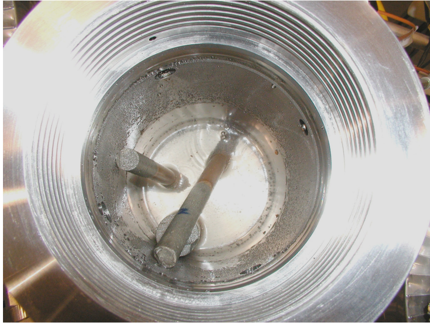
Figure S2. Looking inside one of the high-pressure vessels following a CO 2 sequestration experiment with hardened cement samples in place.
