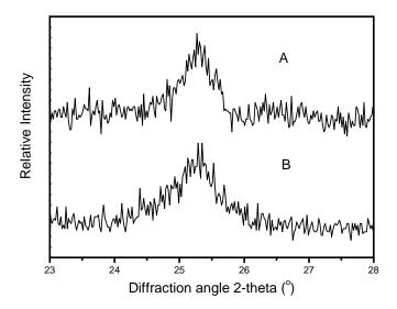
X-ray diffraction peak of crystal plane (101) of the  $TiO_2$  film coated on A  $SiO_2$ -precoated ceramic tile; B ceramic tile.
