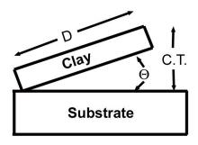
**Supplemental Figure 1.** Given a clay platelet 30 nm in diameter (D) and a multilayer cycle thickness (C.T.) of 47 Angstroms (4.7 nm), a single clay platelet may tilt by  $\Theta$ , 9°. This calculation was performed using Pythagorean theorem where 30 nm is considered the hypotenuse of a right triangle.
