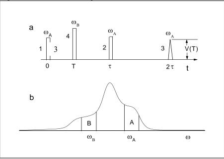
The durations of the first and second pulses forming the spin echo signal were 40 and 70 ns, respectively. The duration of the pumping pulse was 30 ns. The position of the pumping pulse corresponded to the maximum amplitude in the ESR spectrum. The frequency difference was 65 MHz.
