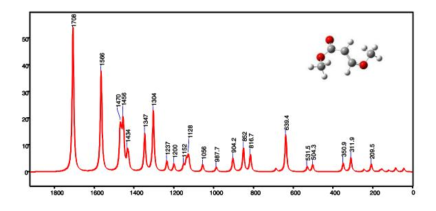
Figure 2: Calculated Raman spectrum of methyl 3-methoxyacrylate (species 5 in Scheme I), obtained by using the Gaussian 03 software, where the most intense features are detailed in parenthesis (1708 cm<sup>-1</sup> C=O and C-H stretch, 1566 cm<sup>-1</sup> C=C stretch and delocalized motion over the entire chain, 1470 cm<sup>-1</sup> C-H bending and stretching over the entire chain, 1304 cm<sup>-1</sup> C=C and C=O stretch, C-H bending)
