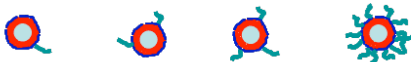
Figure SI-I.6: PEG molecules (drawn in green) are bound to the surface of polymer coated nanoparticles, in a way that 1, 2, 3 PEG molecules are bound per particle or that the particles surface is saturated with PEG.
