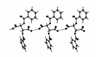
**Figure 7.** Part of one of the chains of hydrogen-bonded anions in the structure of the (-)-5 salt. The spacing along the chain corresponds to the length of the crystallographic b axis.
