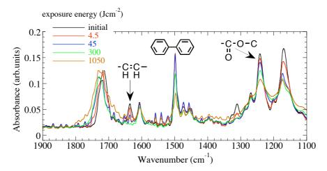
When the exposure energy is until 50 Jcm<sup>-2</sup>, decrease at 1635 cm<sup>-2</sup> (double bond in cinnamate) is observed. For the further exposing, decreases at 1500 cm<sup>-2</sup> (biphenyl groups), and at 1240 cm<sup>-2</sup> (ester C-O-C bond) are detected, which correspond to the photodegradation.
