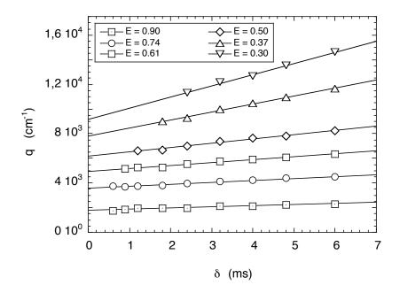
**Figure SI-5.** Lettuce seeds. Plot of experimental values q that generate E(q) = 0.90 ( $\boxdot$ ), 0.74 (O), 0.61 ( $\square$ ), 0.50 ( $\diamondsuit$ ), 0.37 ( $\triangle$ ) and 0.30 ( $\nabla$ ). Linear variations q ( $\delta$ ) are evidenced; q values extrapolated to  $\delta = 0$  are the wave vector magnitudes  $q_{eff}$  in agreement with the SGP approximation.
